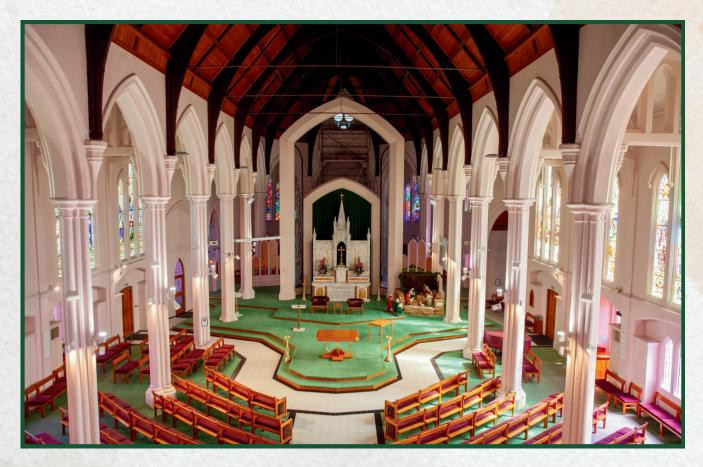
The Cathedral's interior reflects a refined, unadorned Gothic style, marked by soaring arches and a sense of majesty. Fourteen fluted white concrete columns rise to 22 feet, supporting the vast roof structure above. These columns are reinforced with steel from foundation to peak, speaking to the strength and permanence of the design.
